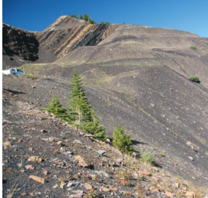
The east side of Grassy Mountain was lined with un-reclaimed dirt slopes. Slumping had occurred in several spots where access fluid from drilling had flowed down into the valley below. Photo © D. MAYHOOD
